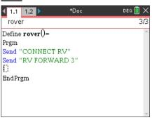
Use the arrow keys to position the cursor to change the value of the forward distance.
